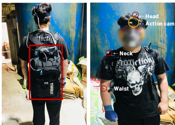
Figure 1. Measurement of PM 10 using direct-reading instrument
