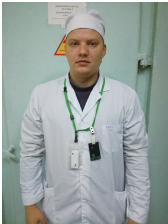
Fig. 9. On-body location of D-Shuttle and Harshaw 6600 dosimeters during exposure.
