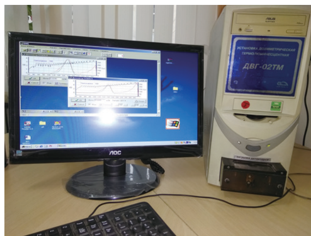
Fig. 1. DVG-02TM, the system for the individual monitoring of ionizing radiation.
