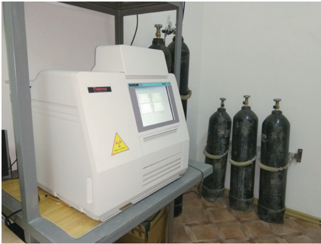
Fig. 2. Harshaw 6600, the system for the individual monitoring of ionizing radiation.
