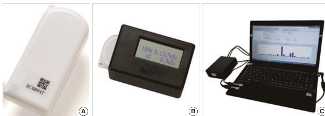
Fig. 6. D-Shuttle dosimeters and their peripheral equipment. (A) D-Shuttle dosimeter, (B) handy indicator, (C) dedicated workstation.
