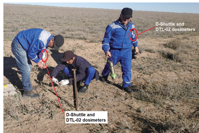
Fig. 12. Location of D-Shuttle and DTL-02 dosimeters on the body during exposure.
