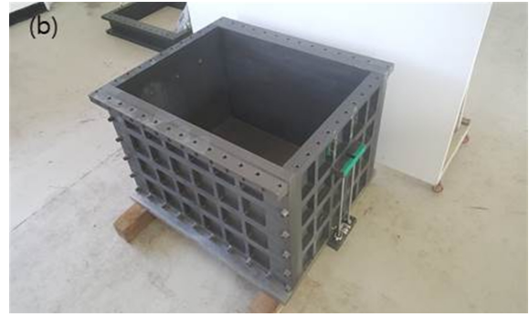
Fig. 1. Soil box (a) Static loading test, (b) Cyclic loading test
