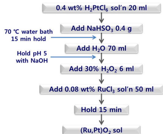
Fig. 3. Preparation of (Ru,Pt)O 2 colloid
