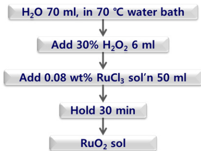
Fig. 4. Preparation of RuO 2 colloid
