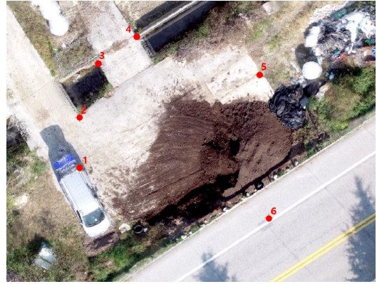
FIGURE 4. Position of tie points
