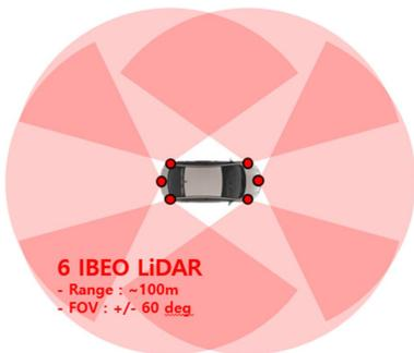
Fig. 2 Detection area of 6 LiDAR (Bird eye view)
