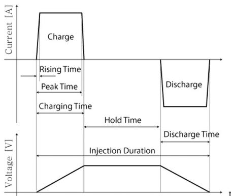
Fig. 1 Driving current wave of piezo injector
