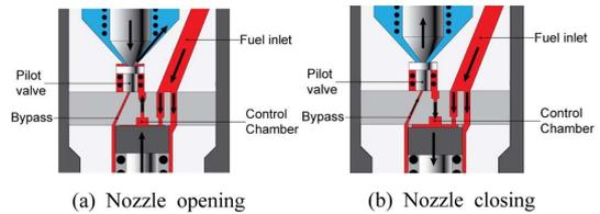
Fig. 2 Nozzle opening/closing stage of piezo injector
