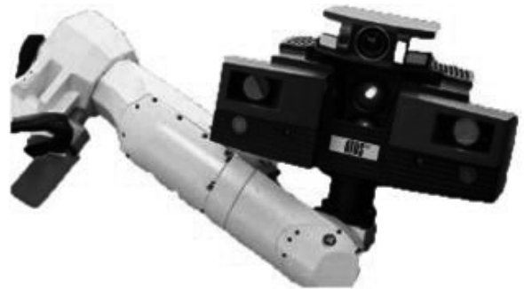
Figure 4. CMM used in this study (ATOS plus, Gom, Germany).
