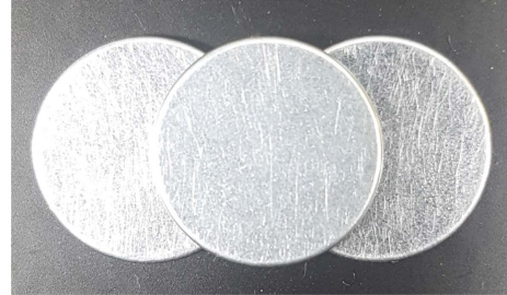
Fig. 1. Waste rare earth magnet sample used in this study (12.3 mm(d) × 1.45 mm(h)).
