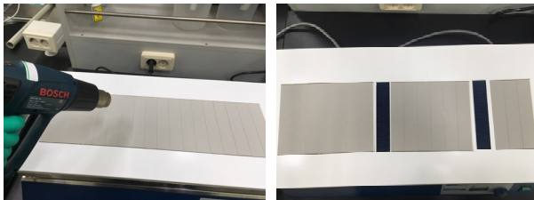
Fig. 6. Pictures for re-work process of shingled string's removal and re-bonding
