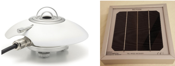
Fig. 6. Pyranometer(left) and Si solar cell(right) type irradiance sensor
