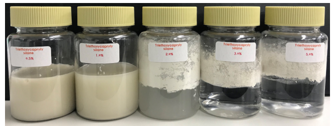
Figure 6. Results of the jadeite powder hydrophobicity test according to the surface modifier content.
