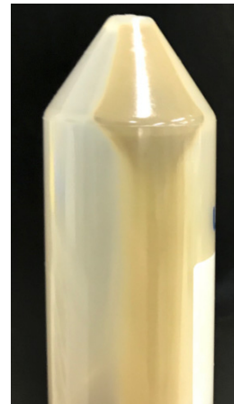
Figure 3. Evaluation standard of oil compatibility test for jadeite powder deposition.
