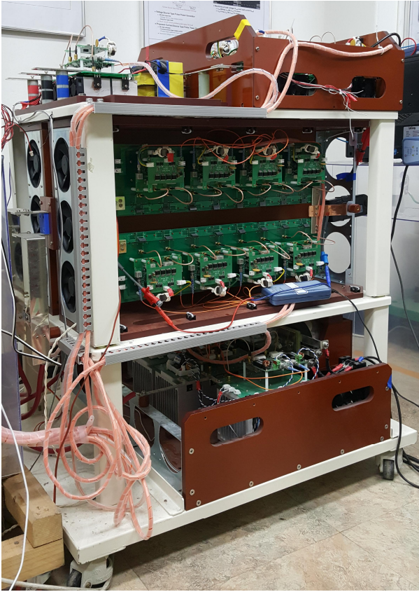
Fig. 10. Experimental setup of current source type pulse generator system.
