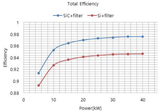
Fig. 10. The comparison of experiment results of Si and SiC inverter of elevator tower system.
