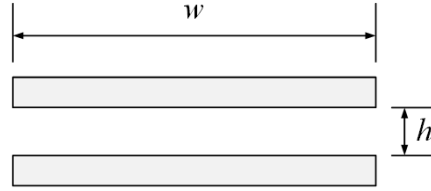
Fig. 1. The structure of DC-link busbar.
