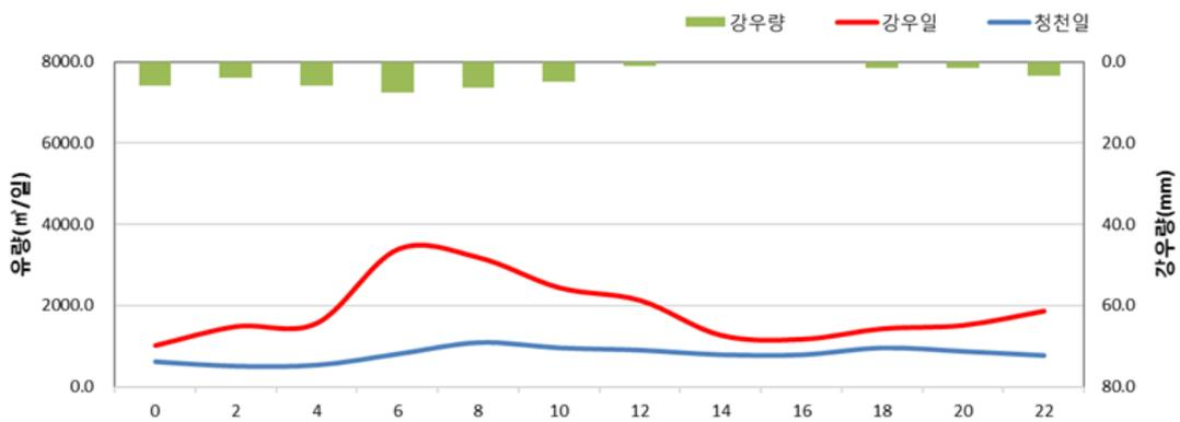
Fig. 10. Curves of flow rate at the same time on the sunny day and the rainy day at point B in AA City (Oct.5,2018)
