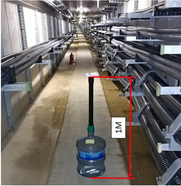
Fig. 3. Measuring of electric and magnetic fields.
