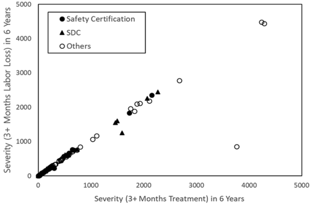
Fig. 8. Relationship between the severity (medical treatment of more than 3 months) and the severity (labor loss of more than 3 months) of the accidents associated with industrial machines and devices in recent 6 years (2012~2017).
