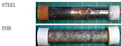
Fig. 9. Galvanic Current Test(3.5% NaCl, 28d)
