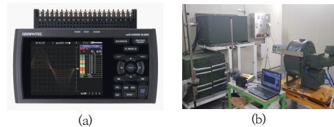
Fig. 8. (a) Data Logger GL820 (b) Temperature Measurement Environment
