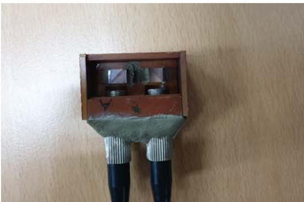
Fig. 3. Fabricated optical current sensor.
