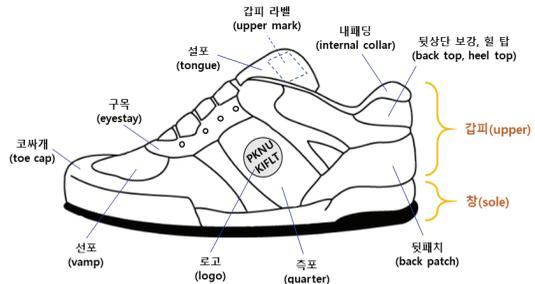
Fig. 2 Structure of shoe
