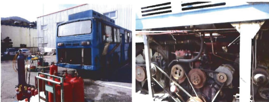
Fig. 3 Experimental testbed Automatic Extinguishing System for vehicle
