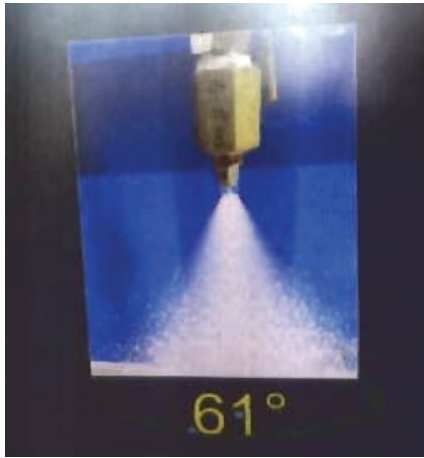
Fig. 6 Experimental results of Spray angle of Spray nozzle
