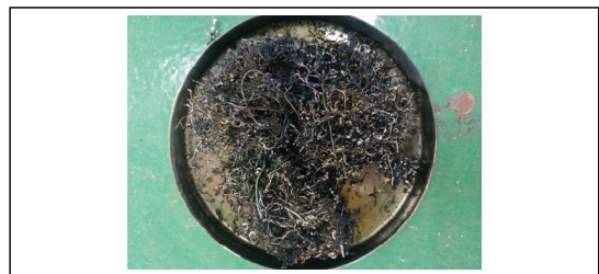
Fig. 8 The photo of burned titanium alloy waste
