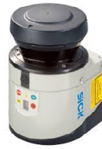
(a) The used laser scanner: LMS 111-10100(SICK)
