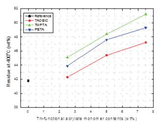
**Figure 7.** Thermal stability of PSA films as a function of tri-functional acrylate monomers.
