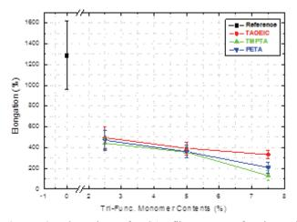
**Figure 6.** Elongation of PSA films as a function of tri-functional acrylate monomers.
