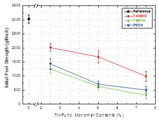
**Figure 3.** Initial peel strength of PSA films as a function of tri-functional acrylate monomers.
