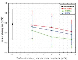
**Figure 9.** Water absorption properties of PSA films as a function of tri-functional acrylate monomers.
