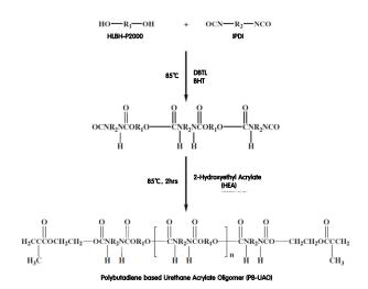
**Figure 1.** Synthetic process of polybutadiene based urethane acrylate oligomer (PB-UAO).
