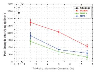
**Figure 4.** Peel strength of PSA films after aging as a function of tri-functional acrylate monomers.
