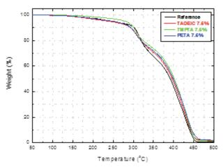
**Figure 8.** TGA graph of PSA films including 7.5 wt% of tri-functional acrylate monomers.
