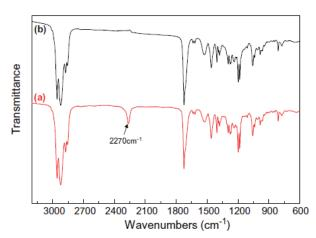
**Figure 2.** FT-IR spectra of synthesized polybutadiene based urethane acrylate oligomer (PB-UAO).
