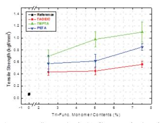
**Figure 5.** Tensile strength of PSA films as a function of tri-functional acrylate monomers.
