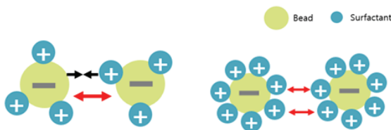
Figure 7. Concept drawing of particle surface charge and inter-particle attraction depending on surfactant contents.
