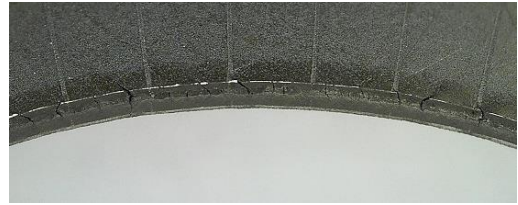
Fig.6 Appearance of edge after hole expansion test
