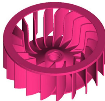
Fig. 2. CAD model of target centrifugal fan.
