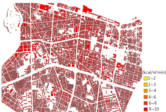
Fig. 6. Emergency power demand of 30 min. of blackout
