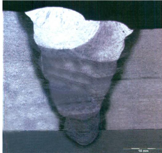
Fig. 12. Welded part macro test result(3G).
