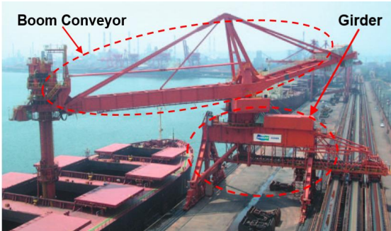
Fig. 1 Continuous ship unloader [5]
