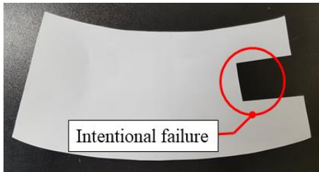
(a) Intentional paper failure for abnormal pressure situation
