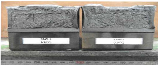
Fig. 6 Fracture surface of 77t-SAW-3
