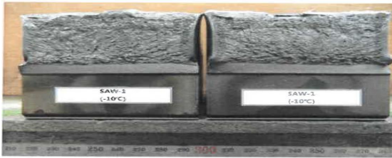
Fig. 4 Fracture surface of 77t-SAW-1
