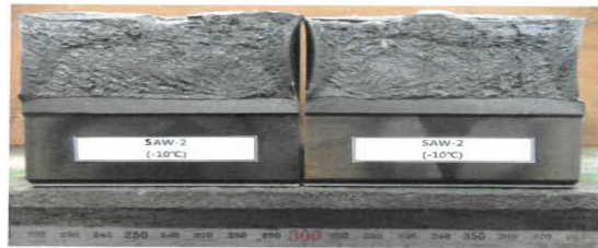
Fig. 5 Fracture surface of 77t-SAW-2
