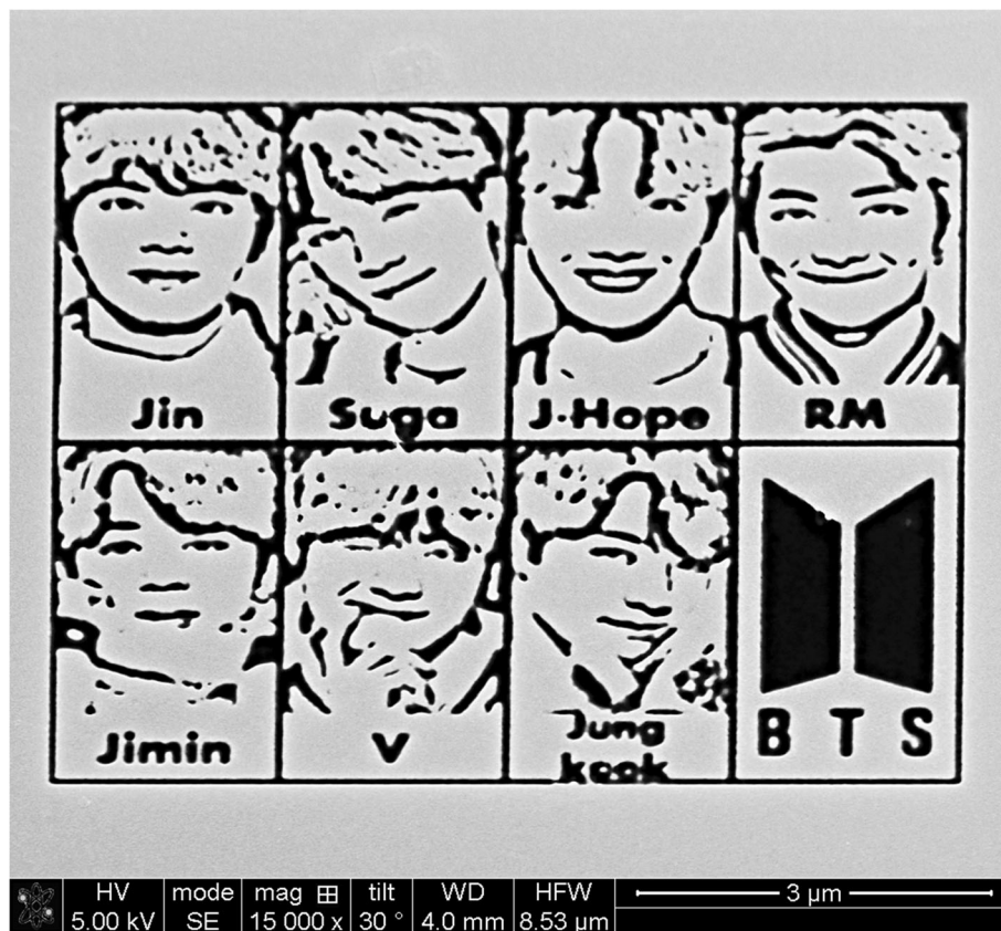
Fig. 1 A SEM image of micro-scale BTS members' portrait patterned by bitmap-assisted patterning function of FIB
