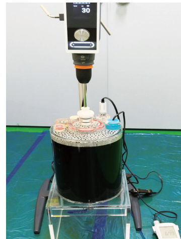
Fig. 3. Practical performance for the selective removal of radioactive ^{137}\text{Cs} from a radioactive liquid waste containing ^{137}\text{Cs} .
