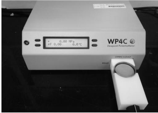
Fig. 1. WP4C equipment for measuring SWCC.
