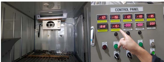
Fig. 9. Unit Cooler Experiment with CO 2 Natural Refrigerant.
