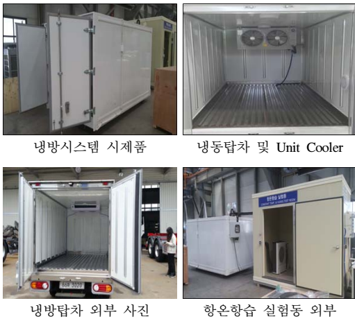
Fig. 10. CO 2 natural refrigerant cooling tower vehicle and prototype.
