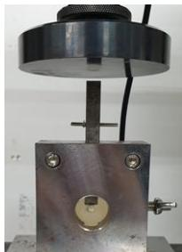
Fig. 2. Experimental setup in the shear bond strength.
