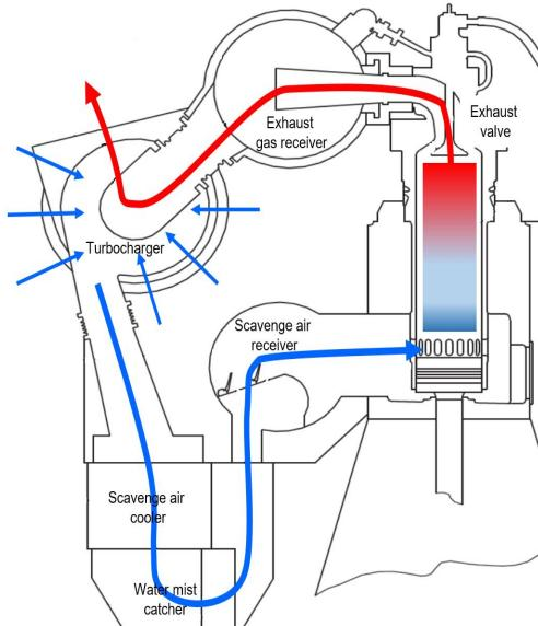
Fig. 3. Exhaust gas system engine
