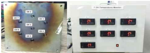
Fig. 7 Temperature measurement sensor and monitoring
