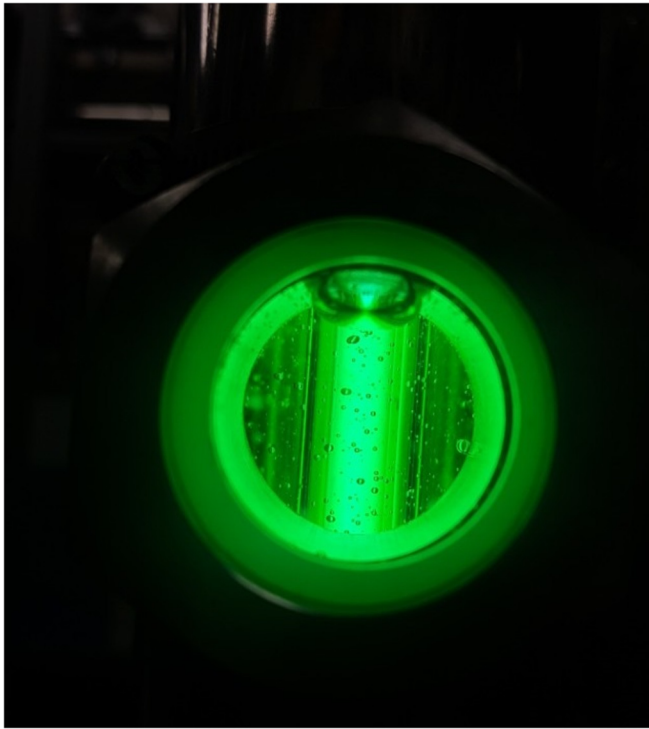
Fig. 3. Image of the vigorous mixing by CO 2 bubbling inside the UVC reactor.
