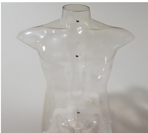
Fig. 1. Torso Mannequin and positions of nanodots for measuring radiation dose.
