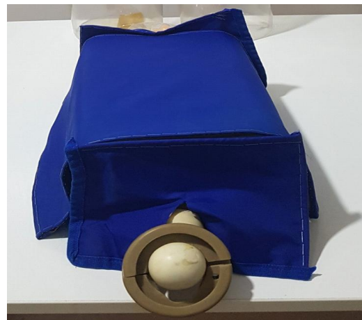
Fig. 2. Shielding device for protection of radiation from arm phantom.
