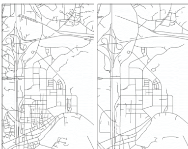
Fig. 3. Road centerline of digital topographic map at 1:5,000 (left) and 1:25,000 (right) scale for target area of training data (all over Giheung-gu, Yongin-si)
