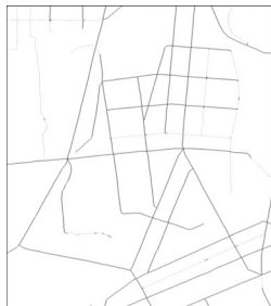
Fig. 8. An example of the discrepancy caused by excessively expressed small road centerlines (the matched line (black) and commission error (gray) of the proposed method)
