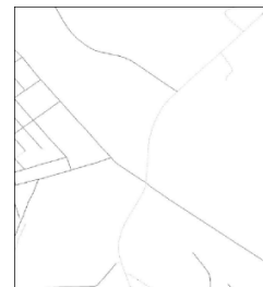
Fig. 6. An example of the discrepancy caused by gaps in the update period (the matched line (black) and commission error (gray) of the proposed method, The vertical road in the middle: a road object that was inserted after renewal of the NGII digital map)
