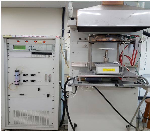
Figure 1. The photograph of cone calorimeter equipment.
