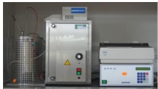
Figure 2. Semiautomatic autoignition tester (ZPA-3).
