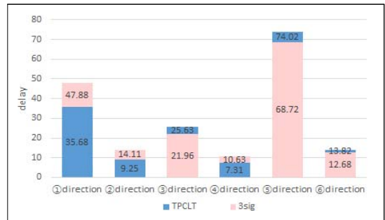
<Fig. 10> Average of control delay by directions when applying the optimization signal and TPCLT signal(Slanting line sections)
