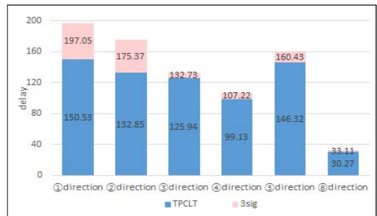
<Fig. 12> Average of control delay by directions when applying the optimization signals and TPCLT signals(Red line sections)
