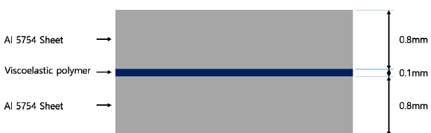
Fig. 1 Schematic of vibration damping aluminum panel applied on this study
