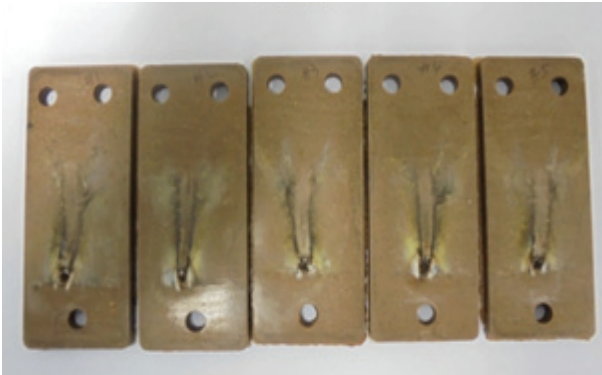
Fig. 2. Vermiculite (10%) tracking test result.
