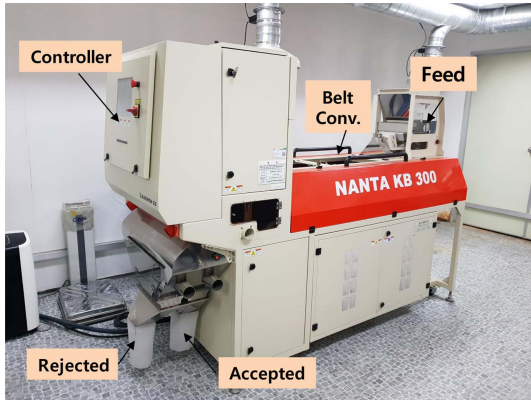
Fig. 4. Photo of the color sorting machine used in the study and component explanation.
