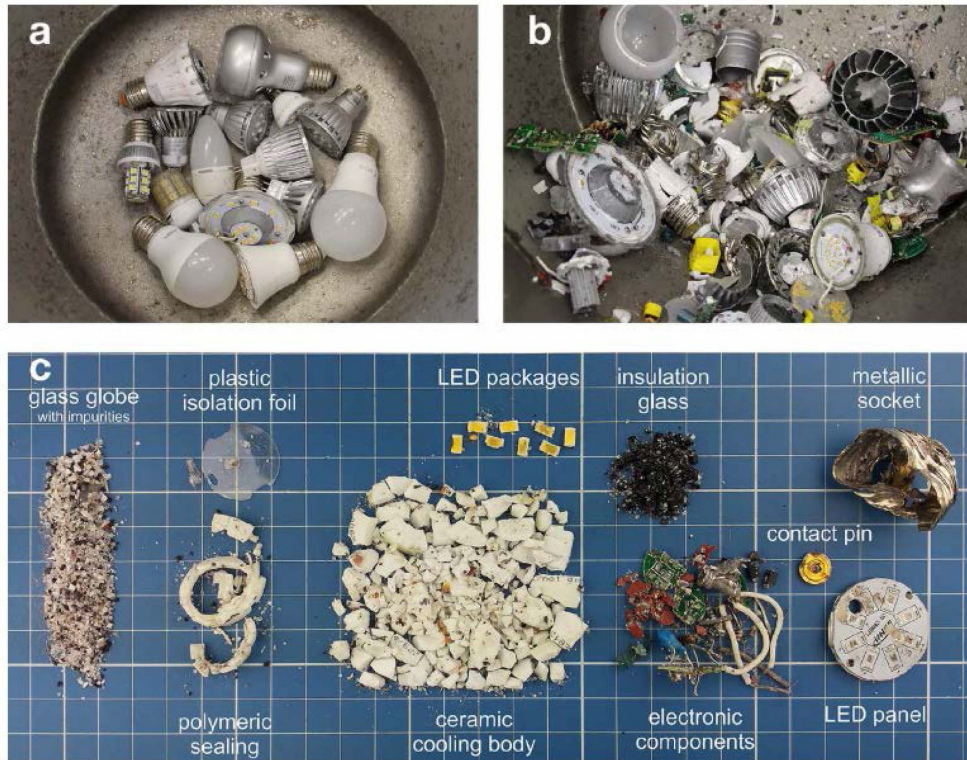
Fig. 4. (a) LED lamp waste, (b) raw material after EHF comminution, (c) separated LED waste component (reprinted from ref. 10).
